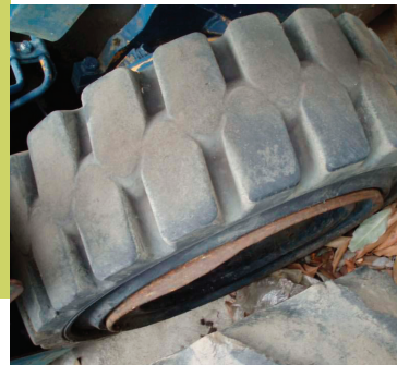
x Unacceptable lock ring damage
