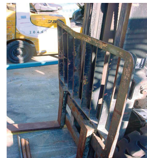
x Unacceptable damage to load guard
