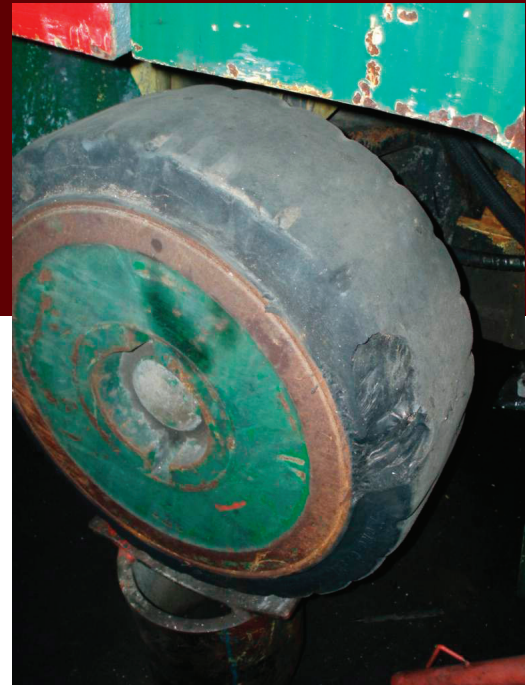
x Unacceptable - Tyre cut
