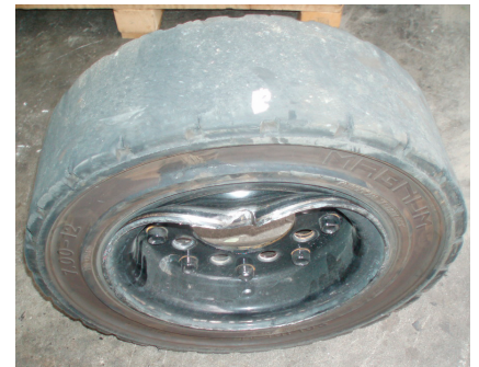
x Unacceptable lock ring damage
