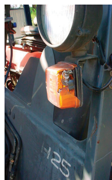
x Unacceptable lens damage
