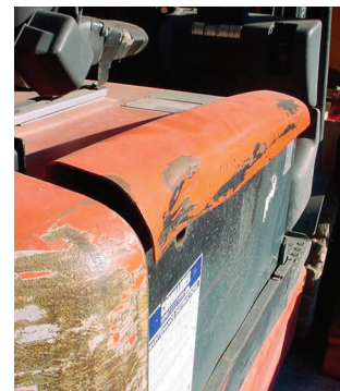
x Unacceptable dents to a battery cover
