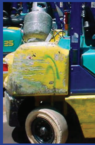
x Unacceptable paint damage
