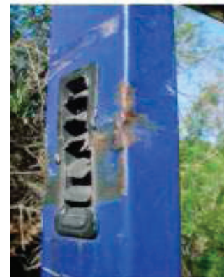
x Unacceptable damage to overhead guard
