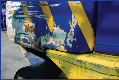
x Unacceptable paint damage
